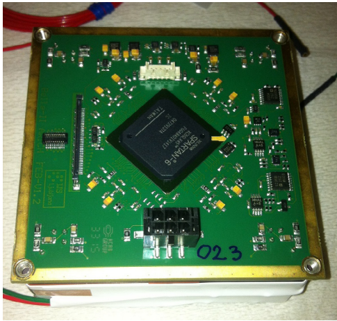
Fig. 1. A photo of the front-end board attached to the HAPD. There are three connectors: one for a data transfer, one for a board power supply and one for a HAPD bias/guard power supply.
