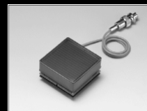
MA-PMT (8 x 8 ch's) Hamamatsu H8500 Active area 49 mm x 49 mm
