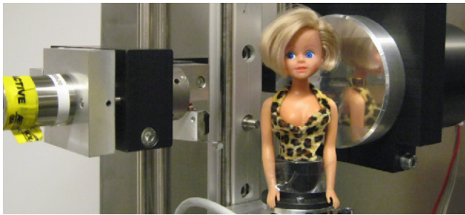
Fig. 1. Photo of KTH-spiralCT. The ^{241}\text{Am} source is in left and the detector is visible behind the doll on the right.
