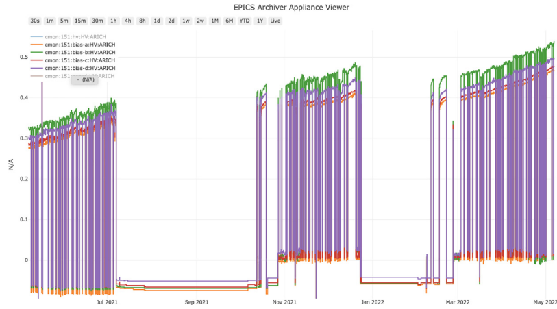
Fig. 3. Monitoring of the bias currents: Due to the irradiation of the sensors, bias currents increase. The time evolution allows to estimate and project the operation usability of the sensors. In this case four bias currents of a particular HAPD are shown as a function of time over a period of about one year. Note that the high voltage is switched off during the detector service. The increase in the current is proportional to the neutron fluence.
