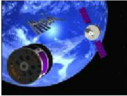
Figure 11: The XEUS X-ray satellite telescope to be launched in 2010. Two separate spacecrafts will simulate a telescope with focal length of 50 m [12].
